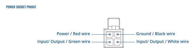
I/O (PIN 3 and 4): Configurable digital Input/Output pins. Open collector output, max output 30 V, 300 mA or Digital input where 0-6 V detected as logic low and 8-30 V – logic high
