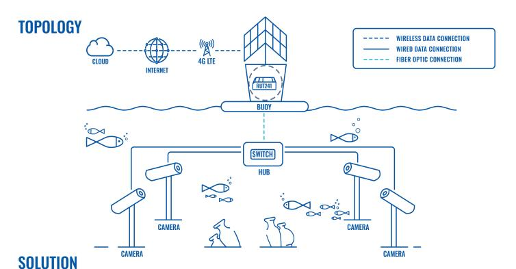
The NOUS system allows continuous monitoring and protection of an underwater site using machine learning and applying image and sound processing algorithms. The system consists of two sections: above and under the water. Onshore or placed on a buoy is a fully autonomous photovoltaic panel system and batteries that provide electricity to the solution. There is also a RUT241 router providing internet via the 4G network, which further travels underwater through the fiber optic cable.
