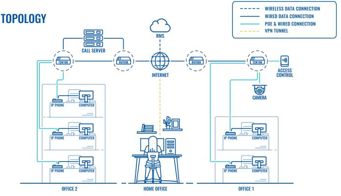
In the headquarters, TSW100 is used to connect the multiple IP phones in the office to the internet and powers them up at the same time, making the setup process very simple and quick. TSW100 switch can power up other devices as well, like IP cameras and Access Control System, as you may notice in the Branch connectivity bit.
