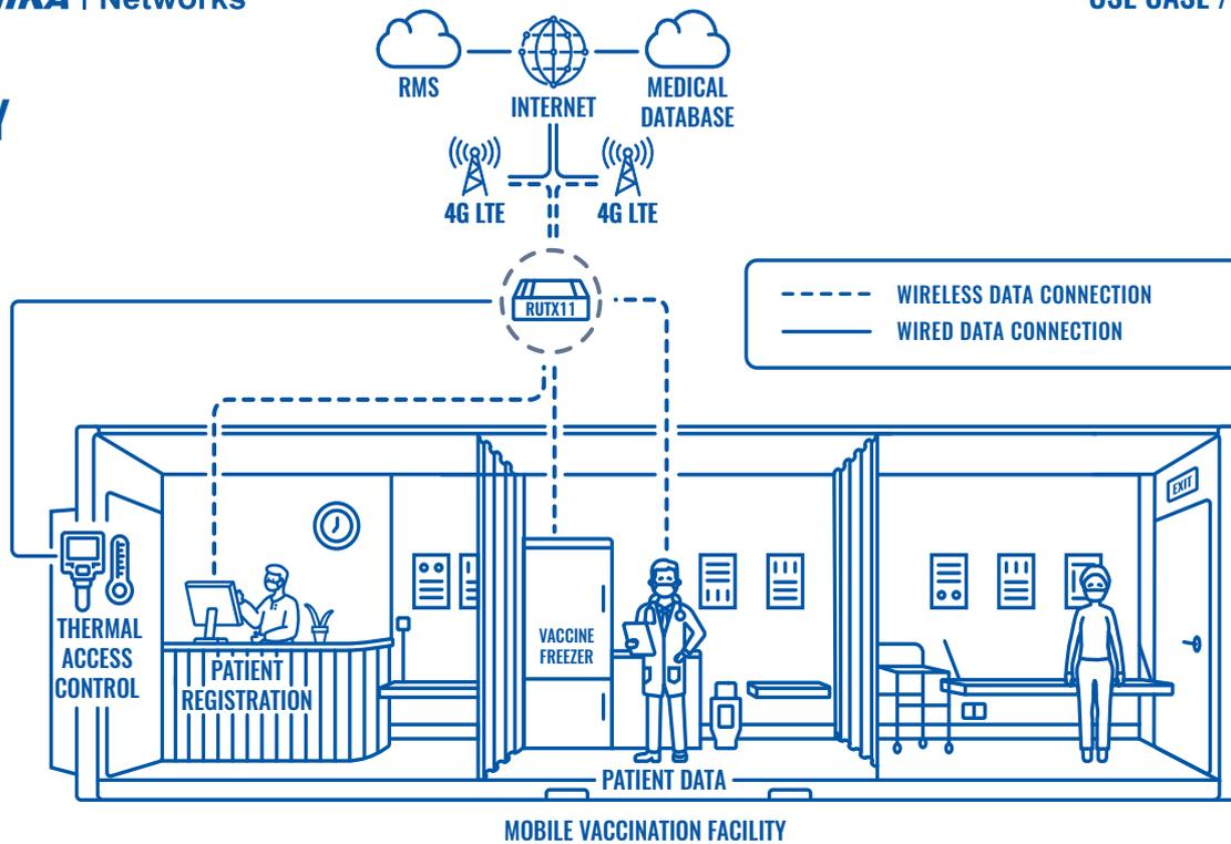
The data from the control unit is sent to the medical database and shared with the reception desk and the medical staff. All of these devices get connected to the network by the RUTX11 - LTE Cat 6 cellular router providing wired and wireless connectivity and ensuring network redundancy with dual SIM functionality.
