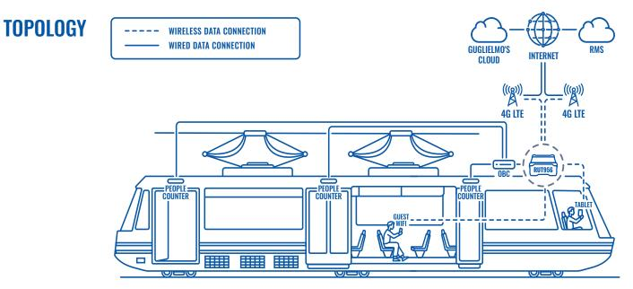
The data is then pushed via MQTT to the Teltonika Networks dual SIM 4G RUT956 router. On the RUT956 MQTT broker, the real-time occupancy data is buffered and provided through a dedicated private WIFI network to the drivers' tablet for monitoring of the passenger flows.
