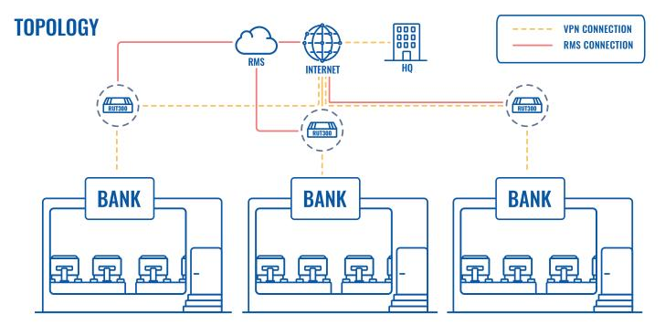
RUT300 Ethernet router has five fast Ethernet ports to easily plug in the computers and gives immediate access to the internet. It is a small device that will easily fit into any cabinet or on a desk and the Passive PoE feature makes it very simple to deploy avoiding additional wires and messy setups. A USB port can be used to easily connect a printer or other office equipment to the network.
