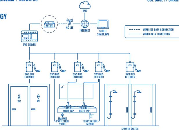
The centrally controlled system maintains water quality in large buildings via fittings and sensors. Operating parameters, like temperatures, or the start and end of a stagnation flush, can be read and evaluated using a data protocol.
