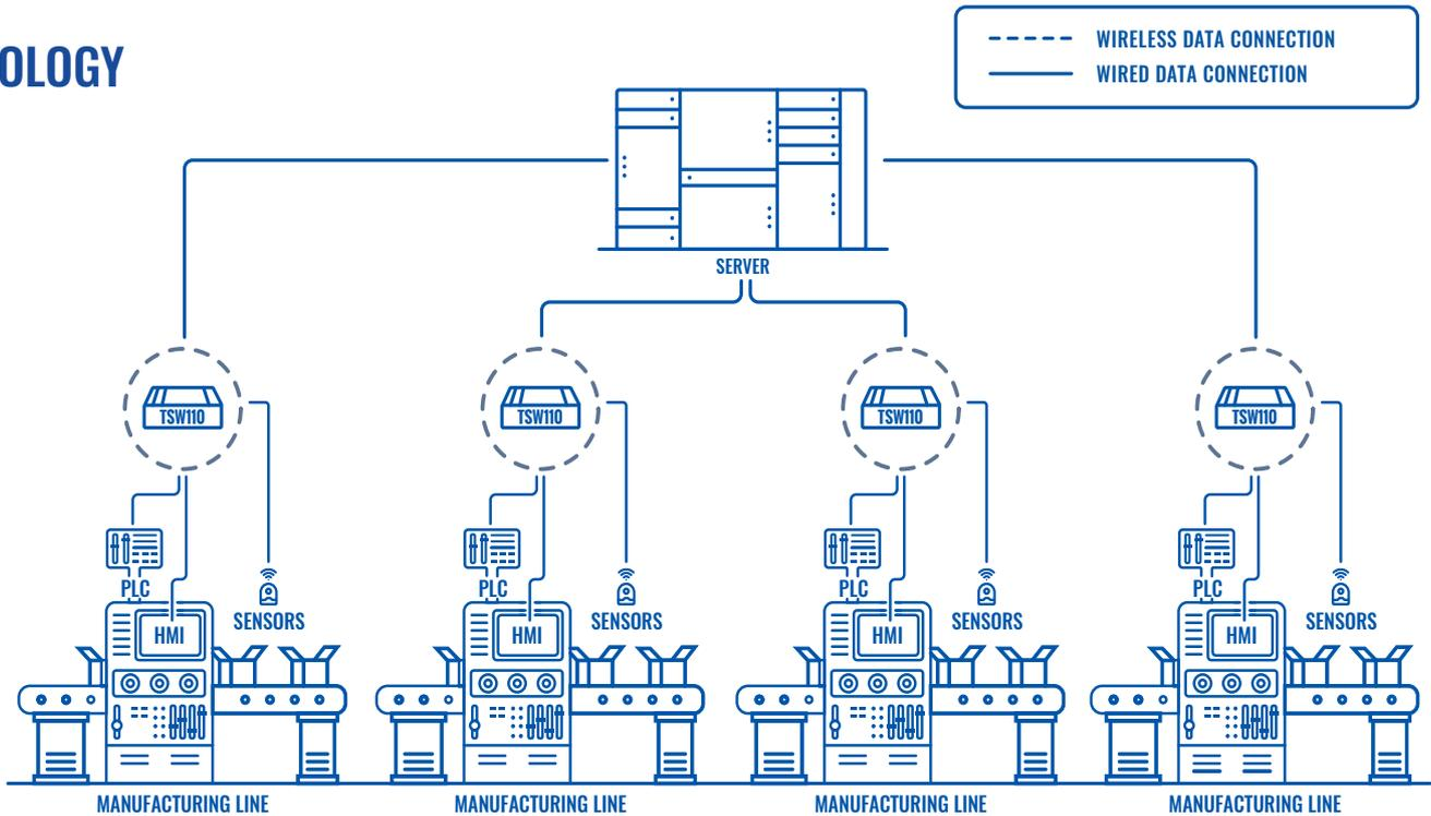
TSW110 is an unmanaged industrial switch with five 10/100/1000 Mbps Ethernet ports for an economical high-bandwidth solution that is more than enough for connecting various manufacturing equipment. Besides, its compact size combined with DIN rail or surface mounting options make it a quick and easy task to deploy it. This plug-n-play device will take seconds to set up!
