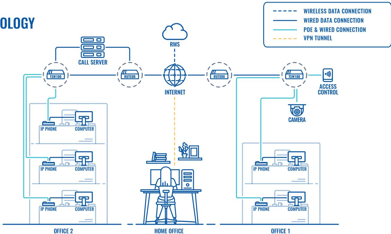
In the headquarters, TSW100 is used to connect the multiple IP phones in the office to the internet and powers them up at the same time, making the setup process very simple and quick. TSW100 switch can power up other devices as well, like IP cameras and Access Control System, as you may notice in the Branch connectivity bit.
